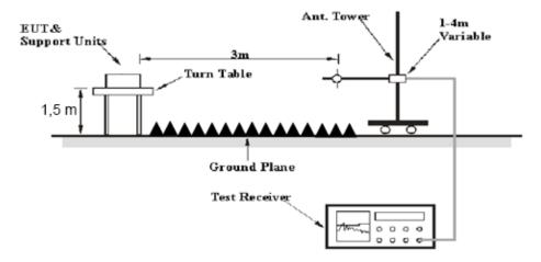
The radiated emission below 1GHz tests were performed in the 3 meters chamber test site A, above 1GHz tests were performed in the 3 meters chamber test site B, using the setup accordance with the ANSI C63.10-2013. The specification used was the FCC 15.209, and FCC 15.249 limits.
