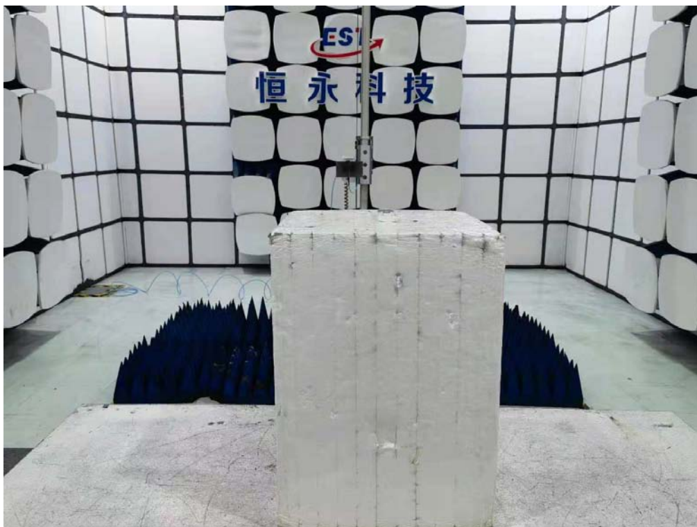
Radiated emission test: Above 1GHz
