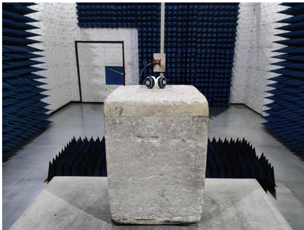
RADIATED EMISSION TEST SETUP ABOVE 1GHz
