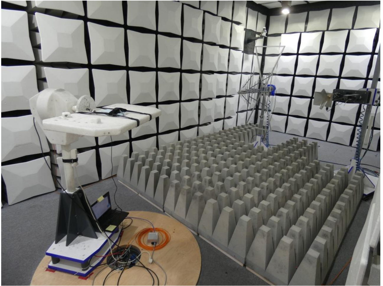
Photo 3: Test setup for radiated measurements (Enclosure, fully-anechoic chamber, 1-26 GHz, intentional radiator §15, ANSI C63.10)
