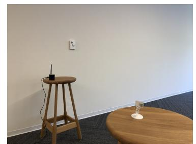
You can apply the tag on top of various surfaces, though please keep in mind that the performance (range, latency) depends on the type of surface. For best results, apply the tag on cardboard or plastic PET material
