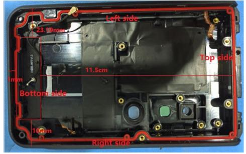
Antenna to Front side 5mm Antenna to Back side 3mm
