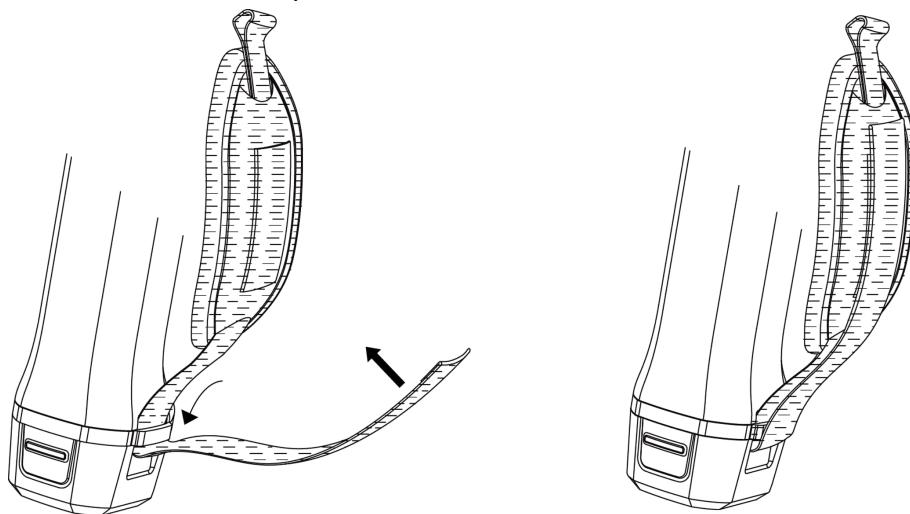
**Figure 2-4 Secure Lower Part of Hand Strap**
