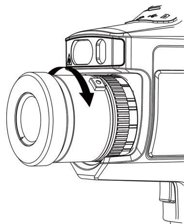
**Figure 2-9 Mount the Teleconverter**
