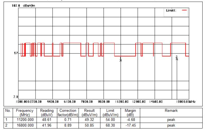
Test Mode: 03; Polarity: Vertical; Modulation:802.11a; Bandwidth:20MHz; Channel:middle
