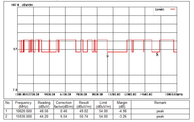
Test Mode: 02; Polarity: Horizontal; Modulation:802.11ac; Bandwidth:40MHz; Channel:High
