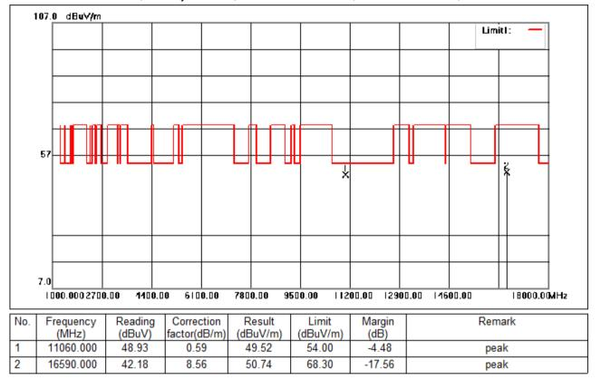
Test Mode: 03; Polarity: Vertical; Modulation:802.11ac; Bandwidth:80MHz; Channel:Low
