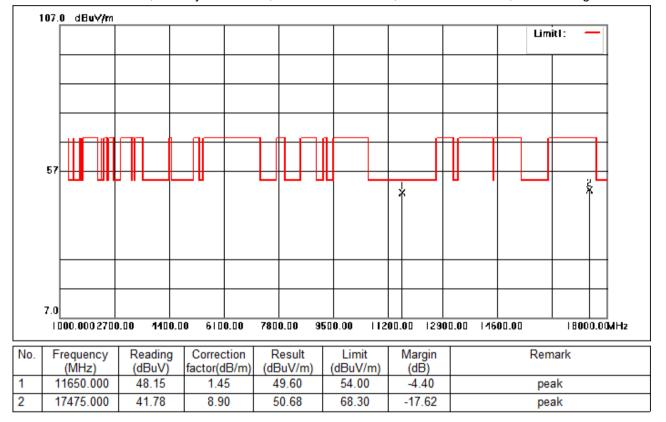
Test Mode: 04; Polarity: Horizontal; Modulation:802.11a; Bandwidth:20MHz; Channel:High
