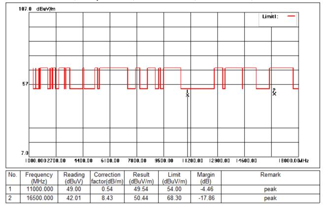
Test Mode: 03; Polarity: Horizontal; Modulation:802.11n; Bandwidth:20MHz; Channel:Low
