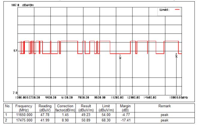
Test Mode: 04; Polarity: Vertical; Modulation:802.11ac; Bandwidth:20MHz; Channel:High
