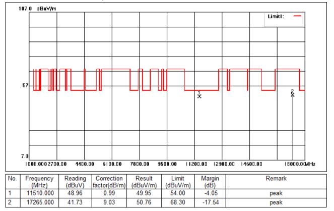
Test Mode: 04; Polarity: Vertical; Modulation:802.11n; Bandwidth:40MHz; Channel:Low
