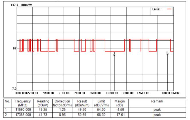
Test Mode: 04; Polarity: Vertical; Modulation:802.11ac; Bandwidth:40MHz; Channel:High
