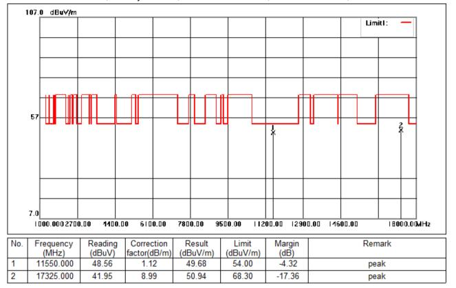
Test Mode: 04; Polarity: Vertical; Modulation:802.11ac; Bandwidth:80MHz; Channel:Low
