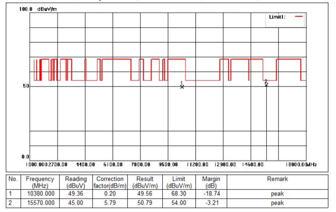
Test Mode: 01; Polarity: Horizontal; Modulation:802.11n; Bandwidth:40MHz; Channel:Low
