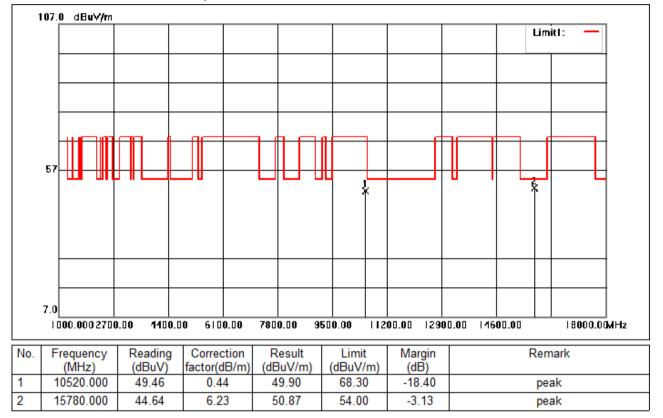
Test Mode: 02; Polarity: Vertical; Modulation:802.11a; Bandwidth:20MHz; Channel:Low
