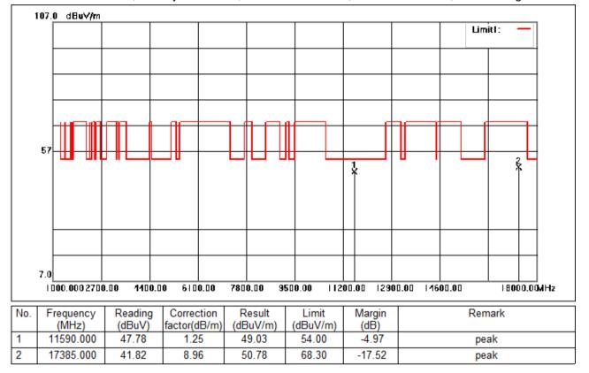
Test Mode: 04; Polarity: Horizontal; Modulation:802.11n; Bandwidth:40MHz; Channel:High
