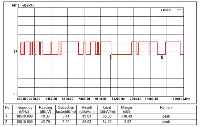
Test Mode: 02; Polarity: Vertical; Modulation:802.11n; Bandwidth:40MHz; Channel:Low
