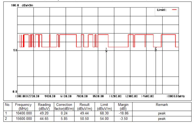
Test Mode: 01; Polarity: Vertical; Modulation:802.11a; Bandwidth:20MHz; Channel:middle
