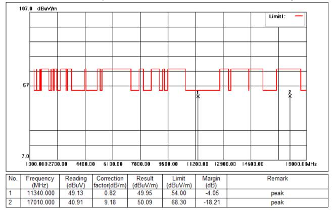
Test Mode: 03; Polarity: Vertical; Modulation:802.11n; Bandwidth:40MHz; Channel:High
