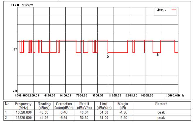
Test Mode: 02; Polarity: Vertical; Modulation:802.11ac; Bandwidth:40MHz; Channel:High
