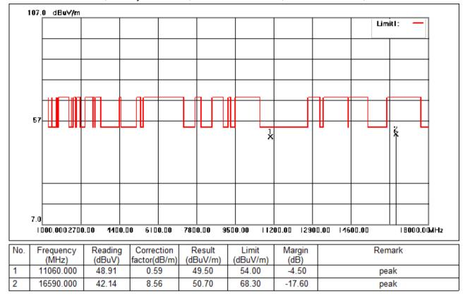
Test Mode: 03; Polarity: Horizontal; Modulation:802.11ac; Bandwidth:80MHz; Channel:Low
