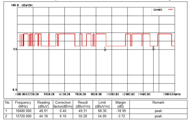
Test Mode: 01; Polarity: Horizontal; Modulation:802.11ac; Bandwidth:20MHz; Channel:High
