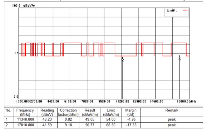
Test Mode: 03; Polarity: Horizontal; Modulation:802.11ac; Bandwidth:40MHz; Channel:High
