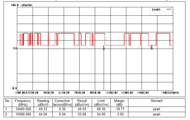
Test Mode: 01; Polarity: Horizontal; Modulation:802.11n; Bandwidth:40MHz; Channel:High
