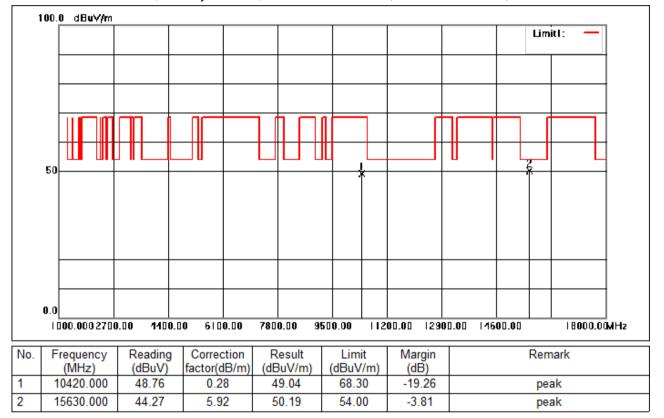
Test Mode: 01; Polarity: Vertical; Modulation:802.11ac; Bandwidth:80MHz; Channel:Low
