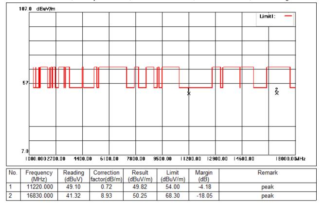
Test Mode: 03; Polarity: Horizontal; Modulation:802.11ac; Bandwidth:80MHz; Channel:High
