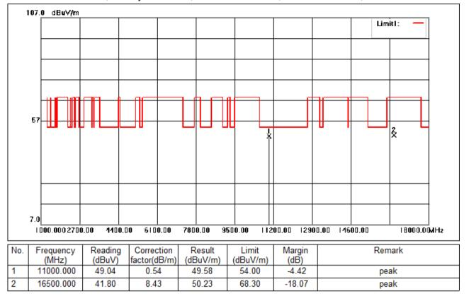
Test Mode: 03; Polarity: Horizontal; Modulation:802.11a; Bandwidth:20MHz; Channel:Low
