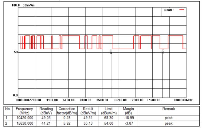
Test Mode: 01; Polarity: Horizontal; Modulation:802.11ac; Bandwidth:80MHz; Channel:Low
