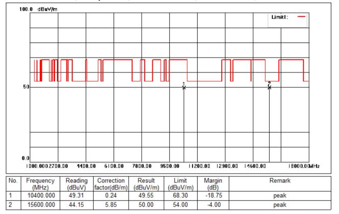
Test Mode: 01; Polarity: Vertical; Modulation:802.11ac; Bandwidth:20MHz; Channel:middle
