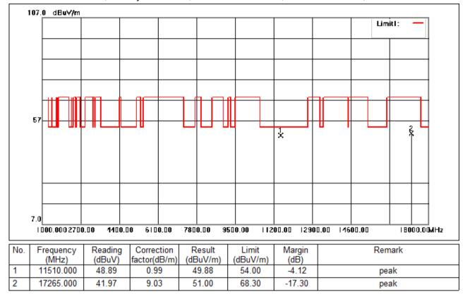
Test Mode: 04; Polarity: Horizontal; Modulation:802.11ac; Bandwidth:40MHz; Channel:Low
