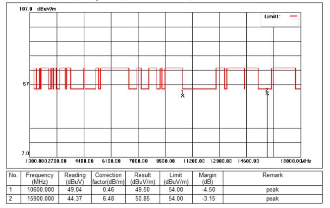
Test Mode: 02; Polarity: Vertical; Modulation:802.11ac; Bandwidth:20MHz; Channel:middle
