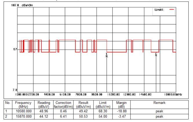
Test Mode: 02; Polarity: Horizontal; Modulation:802.11ac; Bandwidth:80MHz; Channel:Low
