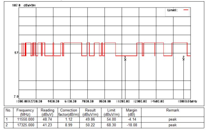
Test Mode: 04; Polarity: Horizontal; Modulation:802.11ac; Bandwidth:80MHz; Channel:Low
