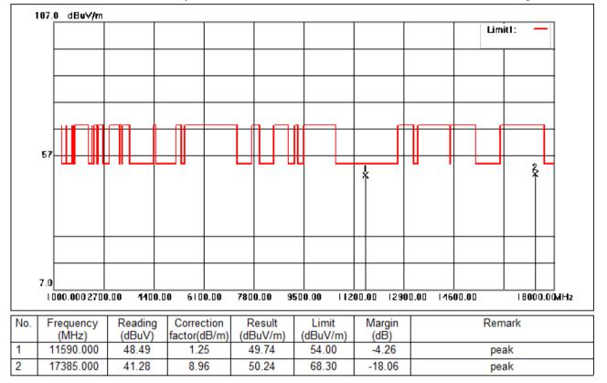
Test Mode: 04; Polarity: Vertical; Modulation:802.11n; Bandwidth:40MHz; Channel:High
