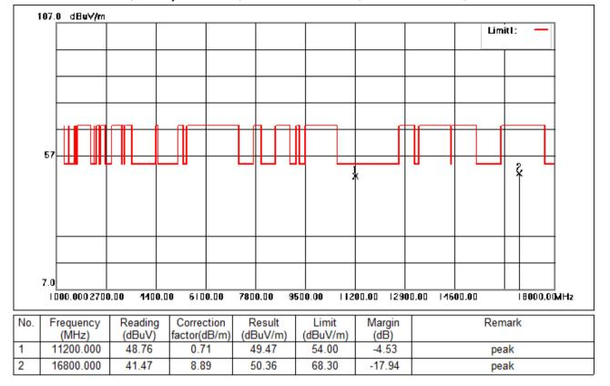
Test Mode: 03; Polarity: Horizontal; Modulation:802.11ac; Bandwidth:20MHz; Channel:middle
