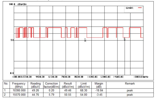
Test Mode: 01; Polarity: Vertical; Modulation:802.11n; Bandwidth:40MHz; Channel:Low
