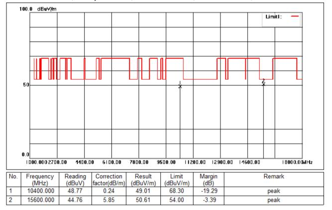
Test Mode: 01; Polarity: Horizontal; Modulation:802.11n; Bandwidth:20MHz; Channel:middle
