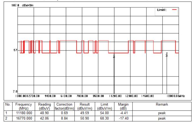
Test Mode: 03; Polarity: Vertical; Modulation:802.11ac; Bandwidth:40MHz; Channel:middle
