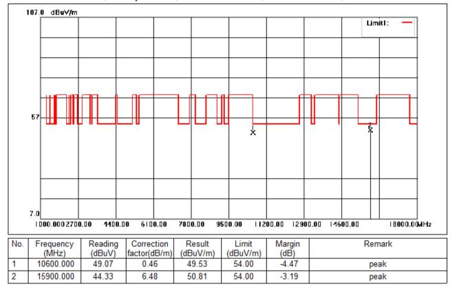
Test Mode: 02; Polarity: Vertical; Modulation:802.11n; Bandwidth:20MHz; Channel:middle
