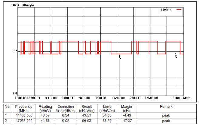
Test Mode: 04; Polarity: Vertical; Modulation:802.11a; Bandwidth:20MHz; Channel:Low
