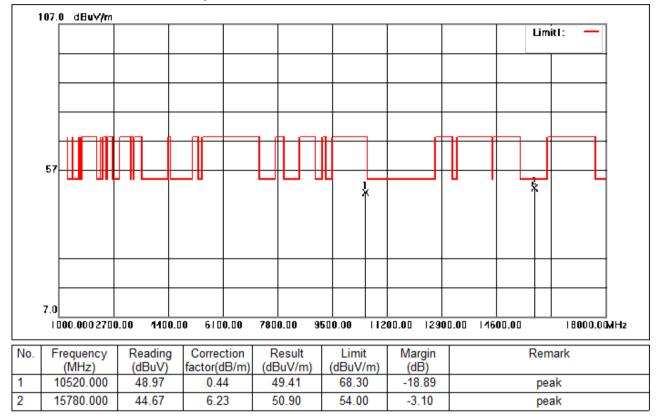
Test Mode: 02; Polarity: Vertical; Modulation:802.11n; Bandwidth:20MHz; Channel:Low
