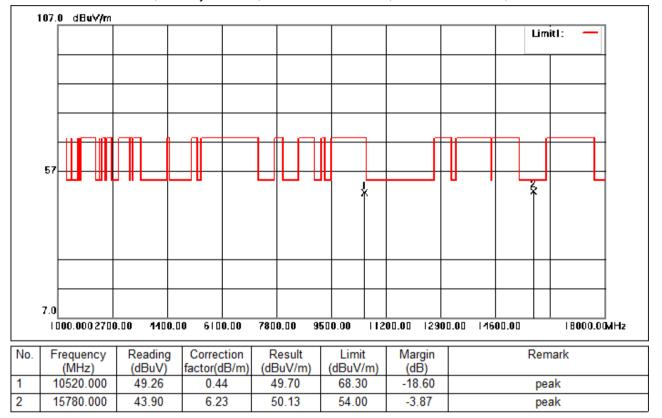
Test Mode: 02; Polarity: Vertical; Modulation:802.11ac; Bandwidth:20MHz; Channel:Low
