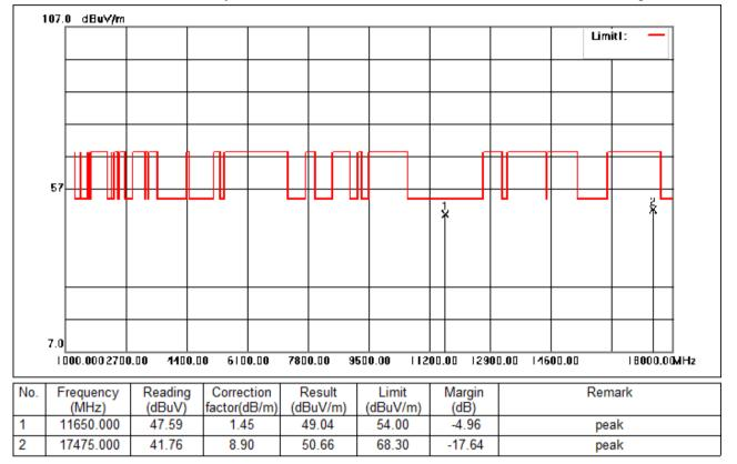
Test Mode: 04; Polarity: Vertical; Modulation:802.11n; Bandwidth:20MHz; Channel:High
