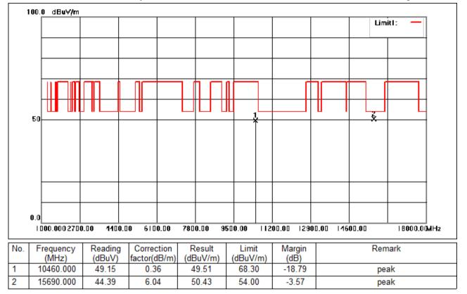
Test Mode: 01; Polarity: Vertical; Modulation:802.11ac; Bandwidth:40MHz; Channel:High
