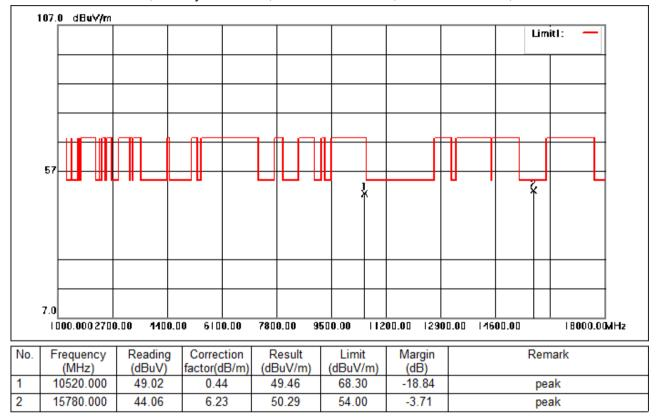
Test Mode: 02; Polarity: Horizontal; Modulation:802.11a; Bandwidth:20MHz; Channel:Low
