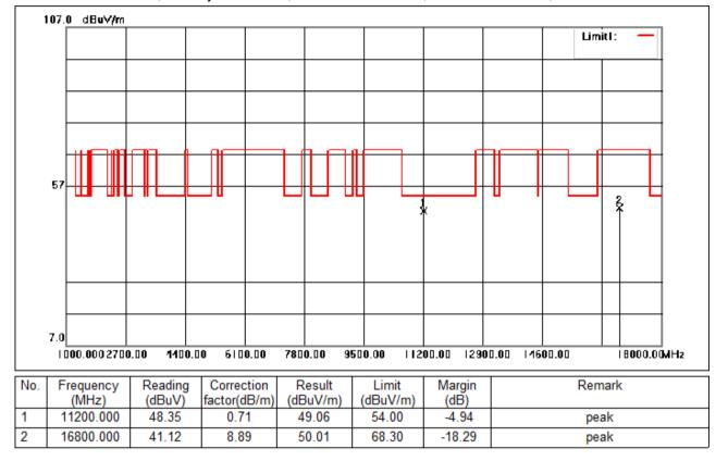
Test Mode: 03; Polarity: Horizontal; Modulation:802.11n; Bandwidth:20MHz; Channel:middle
