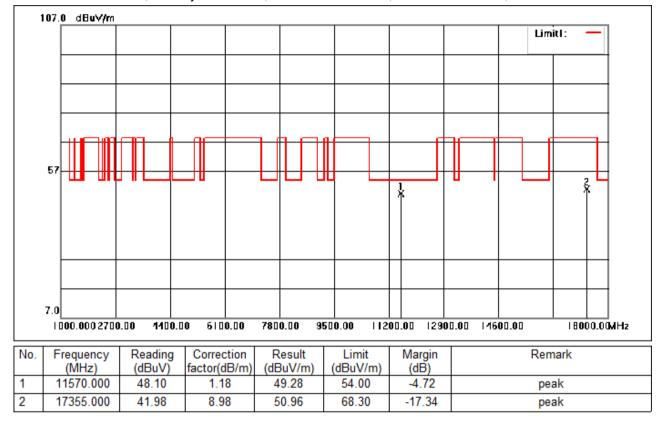
Test Mode: 04; Polarity: Horizontal; Modulation:802.11a; Bandwidth:20MHz; Channel:middle
