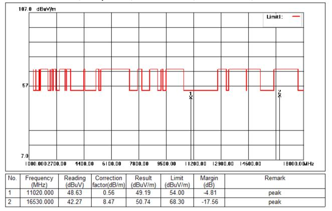
Test Mode: 03; Polarity: Vertical; Modulation:802.11n; Bandwidth:40MHz; Channel:Low
