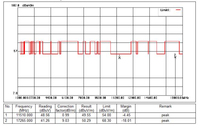
Test Mode: 04; Polarity: Vertical; Modulation:802.11ac; Bandwidth:40MHz; Channel:Low
