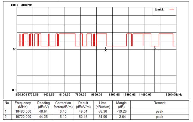
Test Mode: 01; Polarity: Vertical; Modulation:802.11ac; Bandwidth:20MHz; Channel:High
