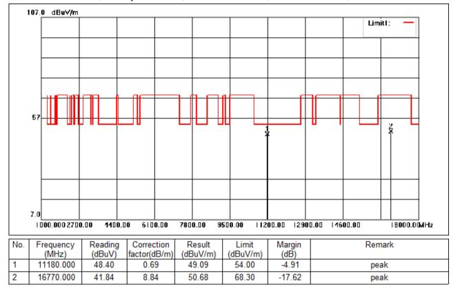
Test Mode: 03; Polarity: Horizontal; Modulation:802.11n; Bandwidth:40MHz; Channel:middle
