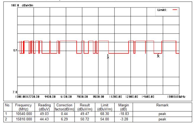
Test Mode: 02; Polarity: Vertical; Modulation:802.11ac; Bandwidth:40MHz; Channel:Low
