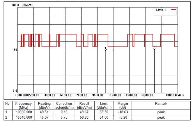
Test Mode: 01; Polarity: Horizontal; Modulation:802.11ac; Bandwidth:20MHz; Channel:Low
