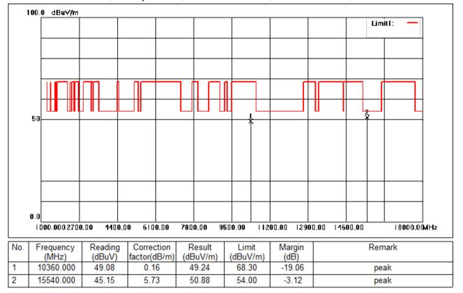
Test Mode: 01; Polarity: Vertical; Modulation:802.11n; Bandwidth:20MHz; Channel:Low
