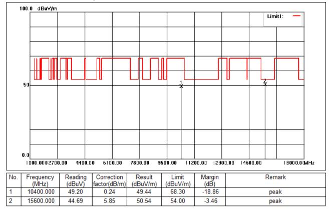
Test Mode: 01; Polarity: Horizontal; Modulation:802.11ac; Bandwidth:20MHz; Channel:middle
