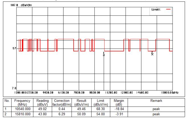
Test Mode: 02; Polarity: Horizontal; Modulation:802.11n; Bandwidth:40MHz; Channel:Low
