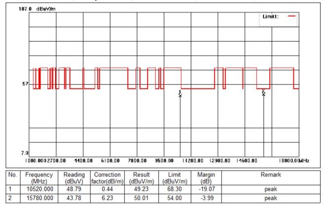
Test Mode: 02; Polarity: Horizontal; Modulation:802.11ac; Bandwidth:20MHz; Channel:Low
