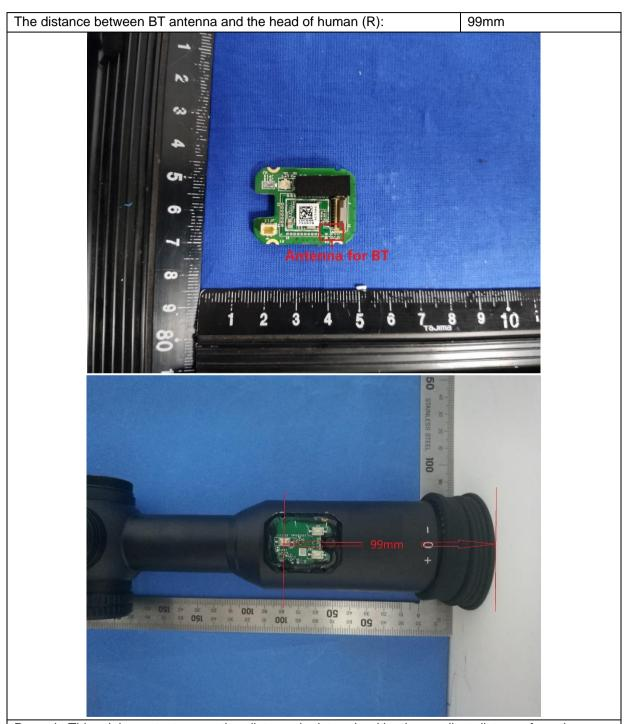
Remark: This minimum test separation distance is determined by the smallest distance from the antenna and radiating structures or outer surface of the device, according to the host form factor,
