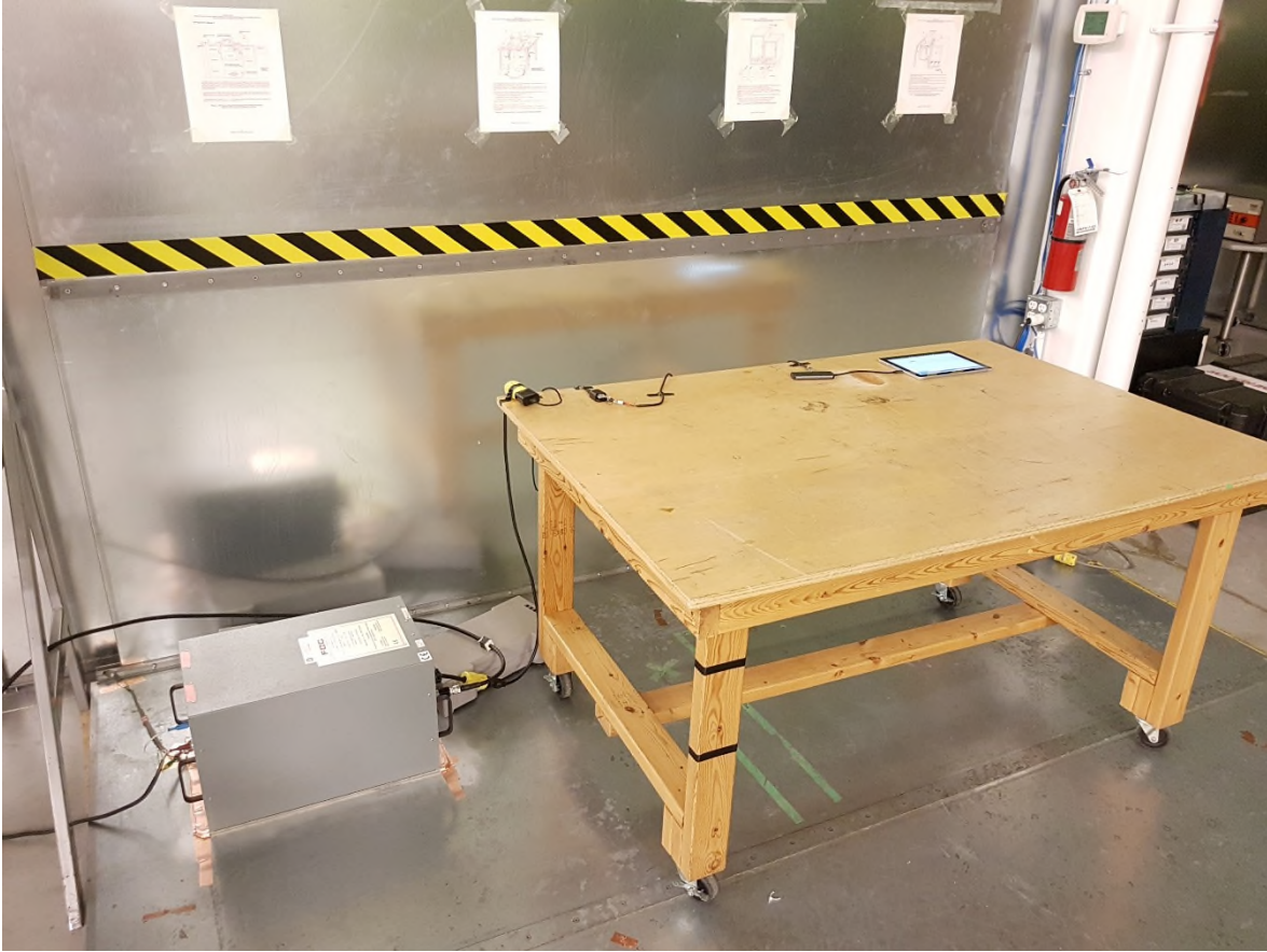
Figure 9 – Conducted Emissions Setup
