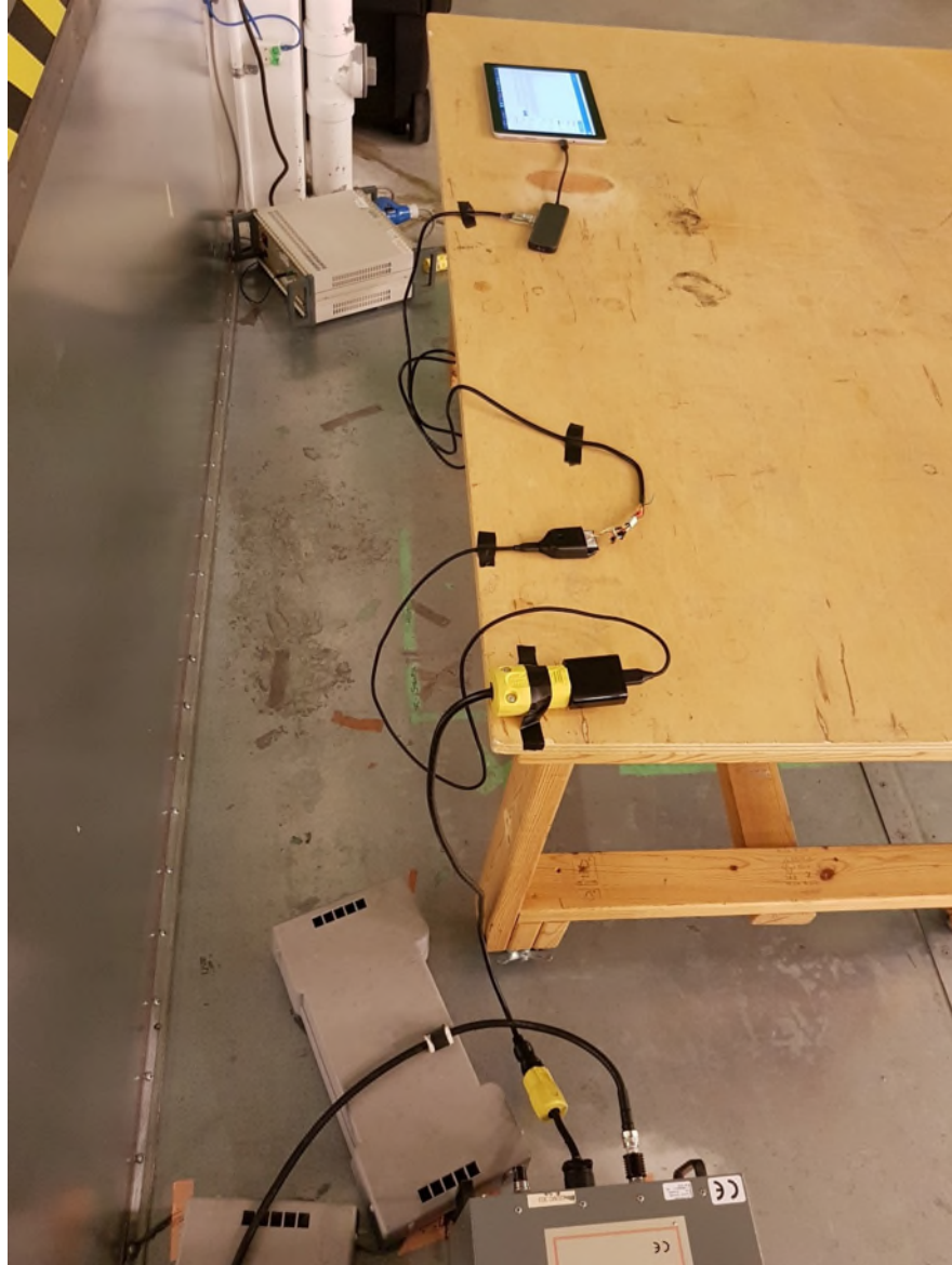
Figure 10 – Conducted Emissions Setup
