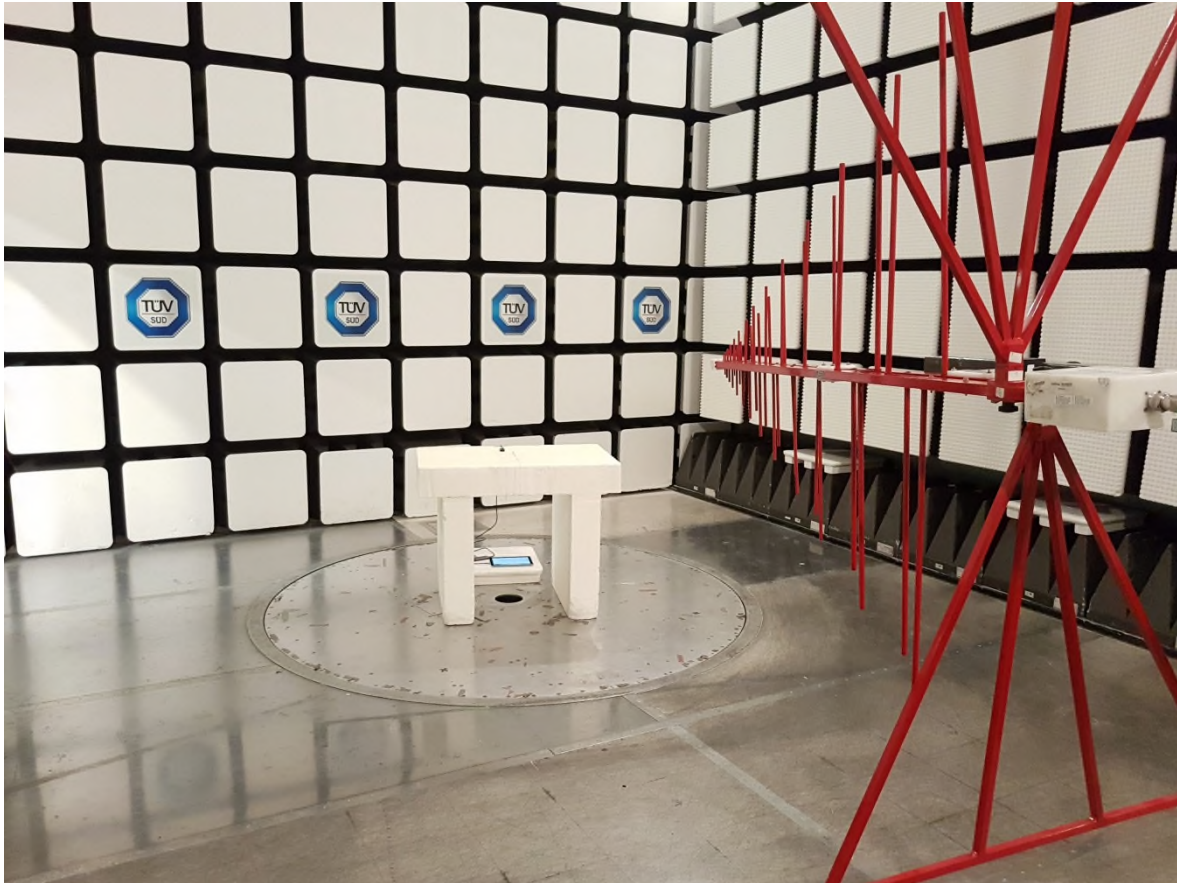
Figure 4 – Radiated Emissions Setup 30MHz to 1GHz
