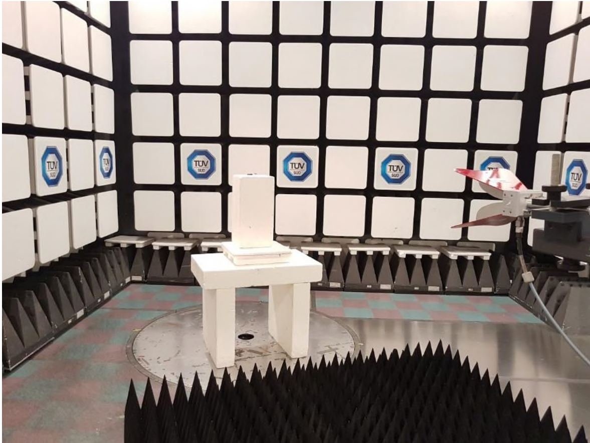
Figure 5 – Radiated Emissions Setup 1GHz to 4GHz Spurious Scans
