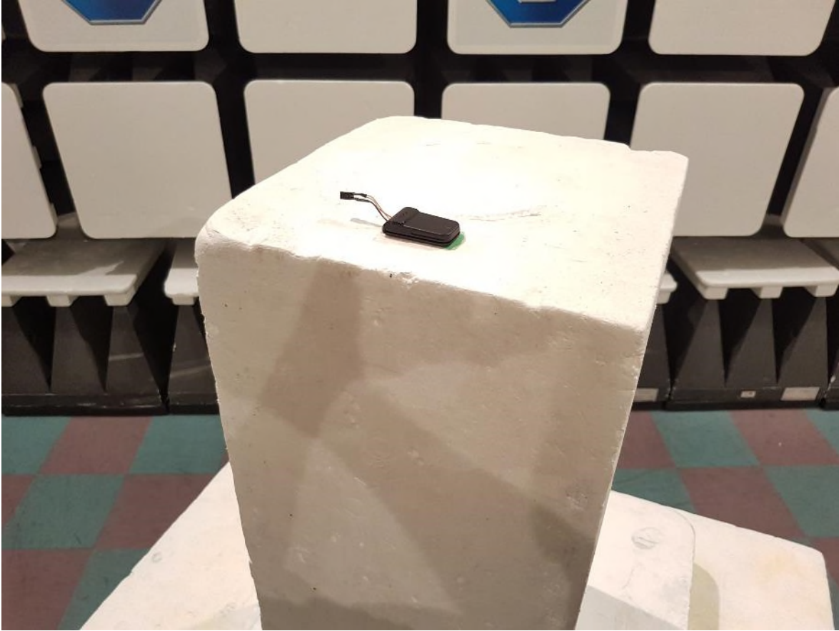
Figure 2 – Radiated Emissions Setup Z-Axis
