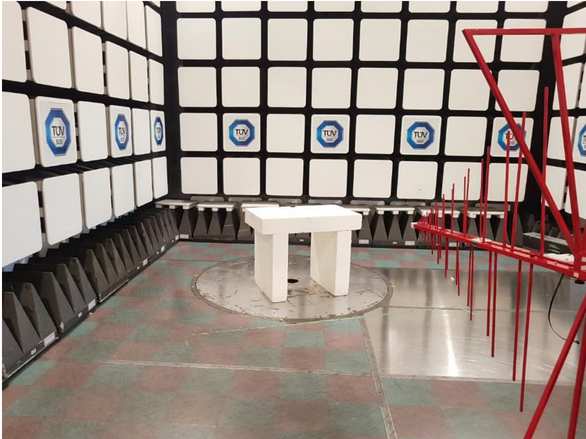
Figure 4 – Radiated Emissions Setup 30MHz to 1GHz
