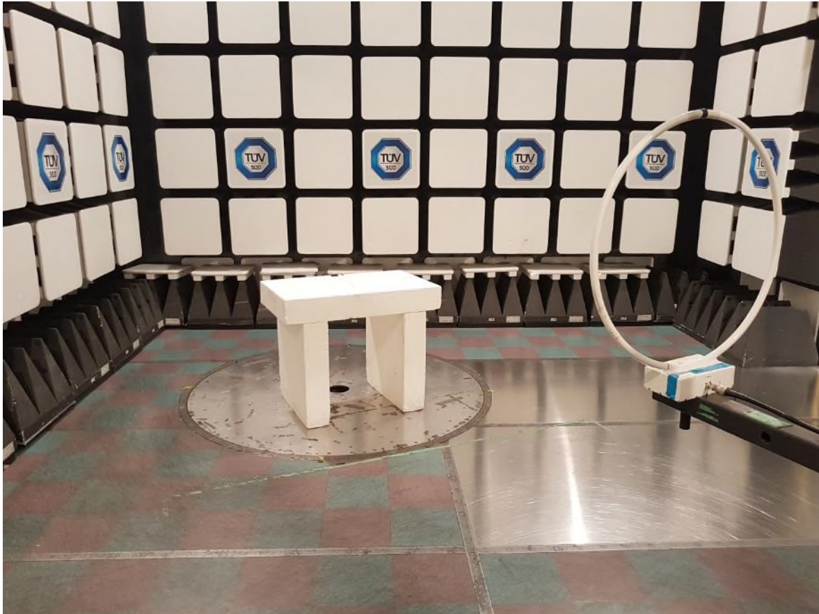
Figure 3 – Radiated Emissions Setup 9kHz to 30MHz
