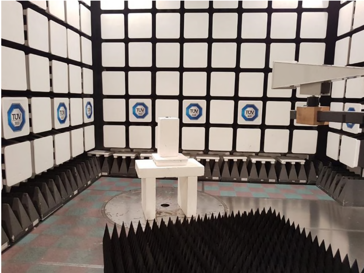
Figure 6 – Radiated Emissions Setup 4GHz to 18GHz Spurious Scans & Band-Edge Measurements
