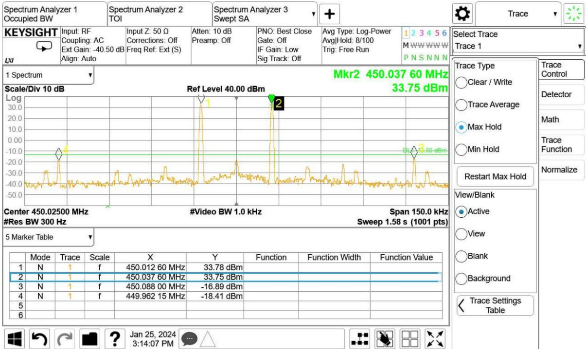
Low Frequency and With the input signal amplitude set 3 dB above the ALC threshold
