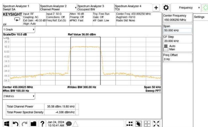
With the input signal amplitude set 3 dB above the AGC threshold Low Frequency: 450.00625MHz
