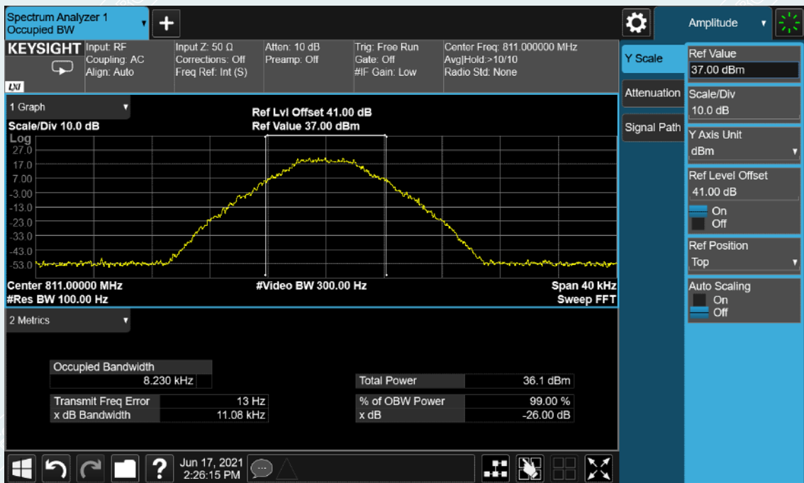
Middle Frequency: 811.0MHz, Output occupied BW (with the input signal amplitude set 3 dB above the AGC threshold)
