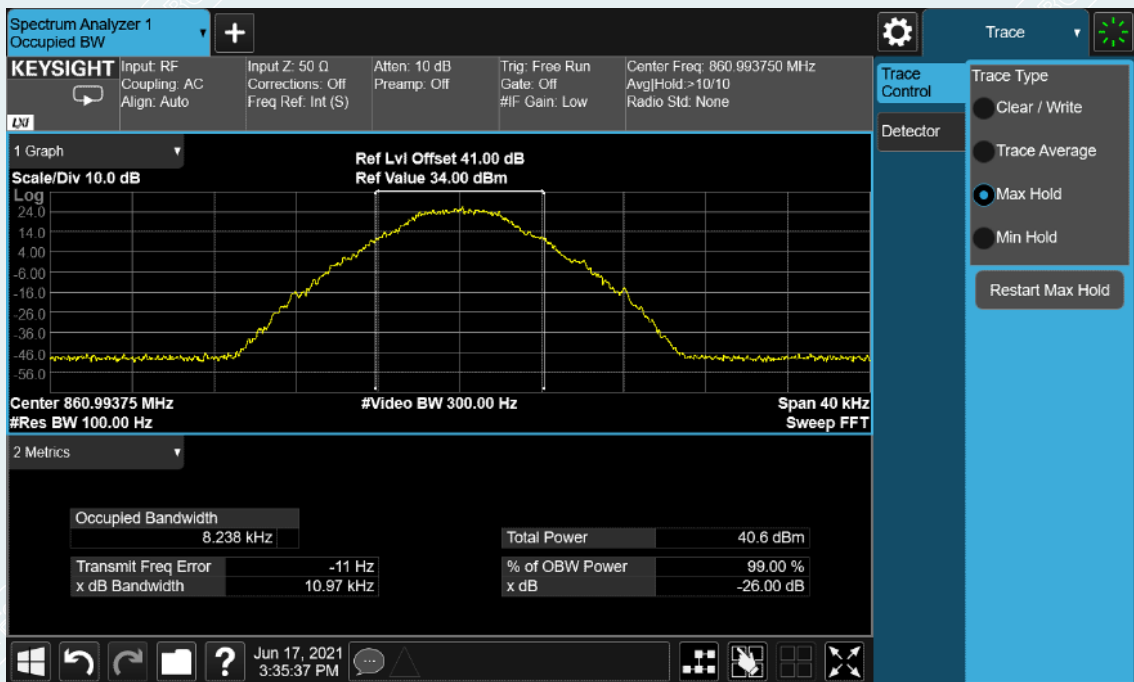
High Frequency: 860.99375MHz, Output occupied BW (with the input signal amplitude set 3 dB above the AGC threshold)
