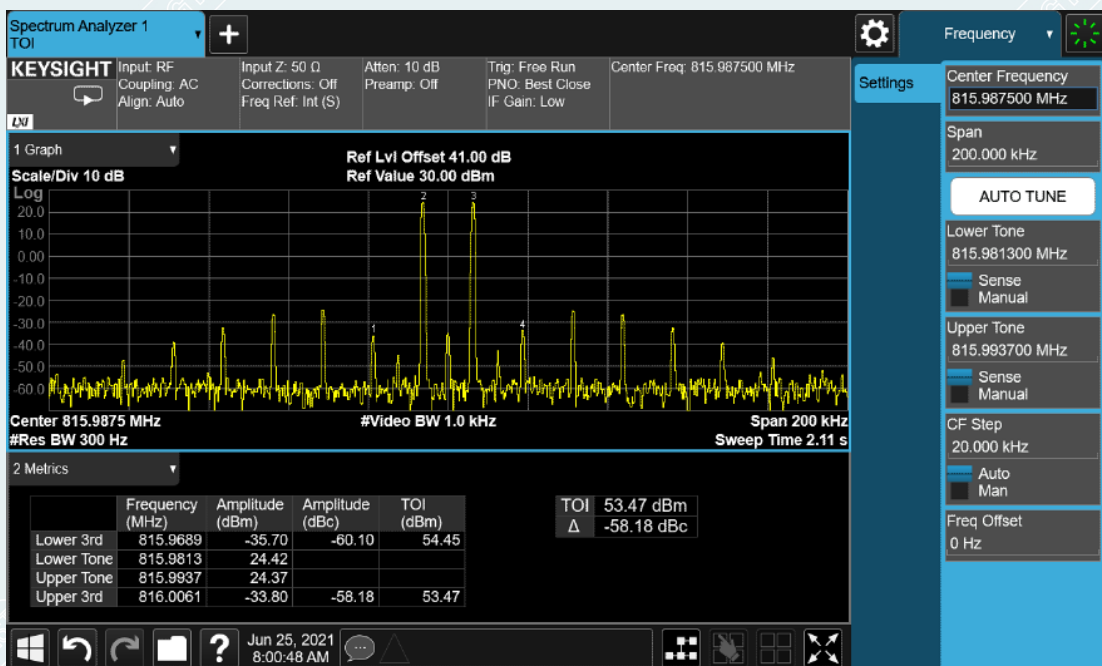
High Frequency and With the input signal amplitude set 3 dB above the ALC threshold
