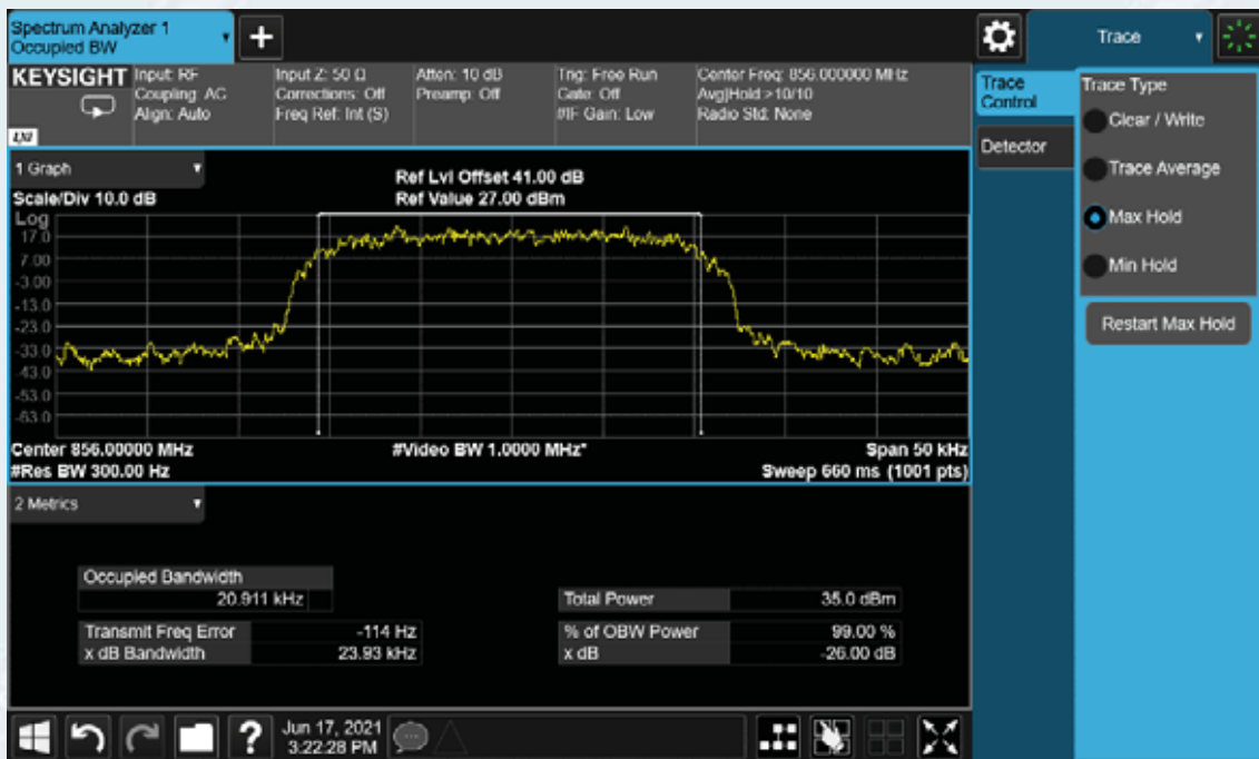
Middle Frequency: 856.0MHz, Output occupied BW (with the input signal amplitude set 3 dB above the AGC threshold)
