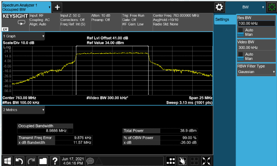
Frequency: 763.0MHz, Output occupied BW (with the input signal amplitude set 3 dB above the AGC threshold)
