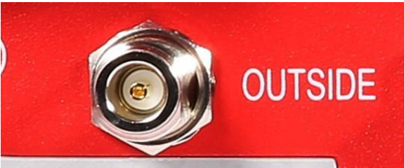
A5— N-type Female for OUTSIDE cable and antenna
