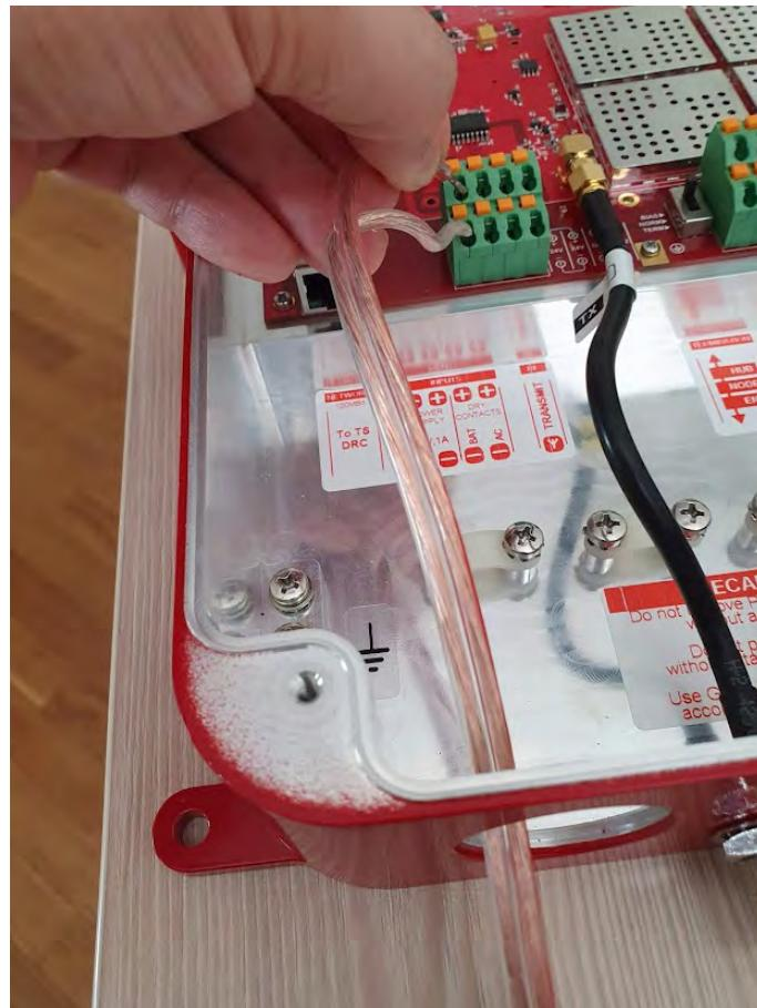
3. Find **X4** 8-pin spring clamp terminal block marked red on the Figure below;
