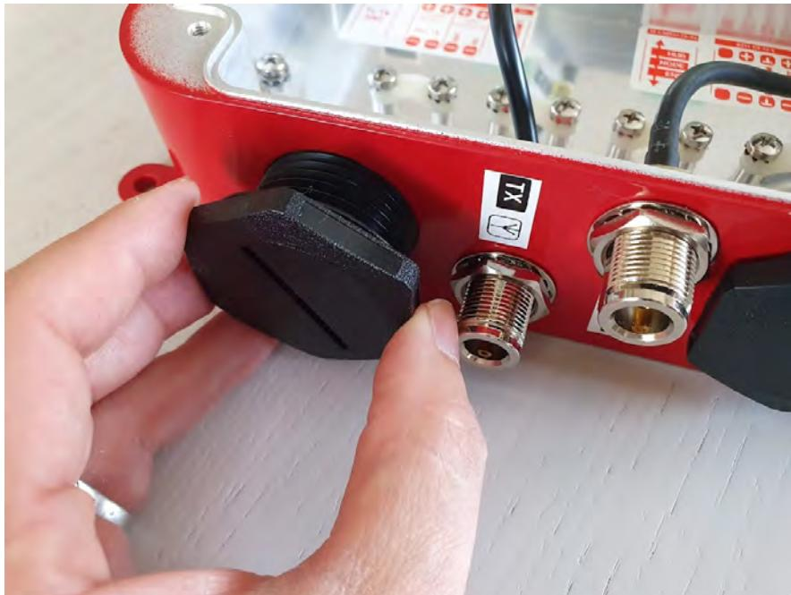
2. Pull power cable through the opening at the bottom of enclosure inside as shown on the following figures.
