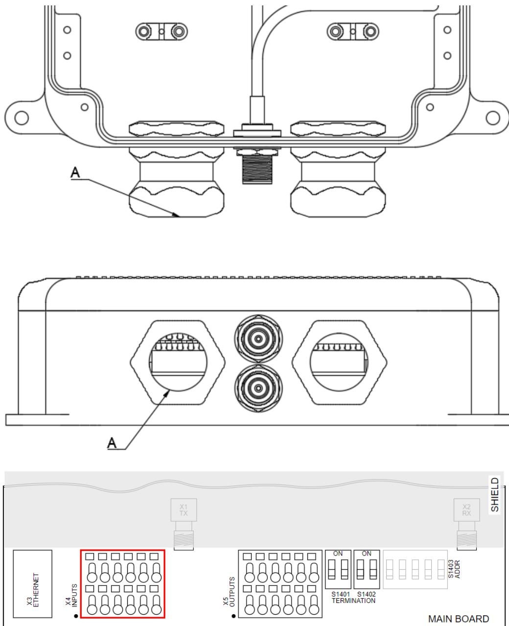
**NOTE:** Terminal block pinout additionally printed in the table on a board surface at the terminal block. It is printed from a left side relatively to spring clamp terminal block.
