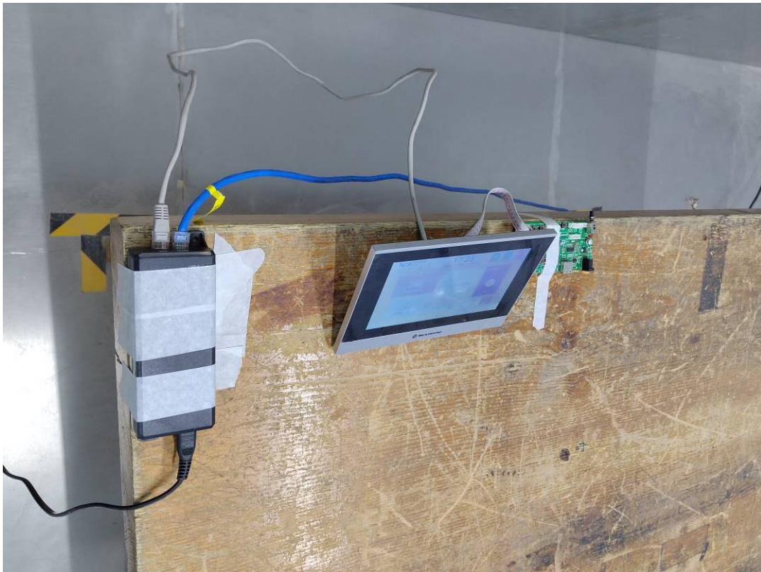
Conducted Emissions Side View- DC power Supply mode
