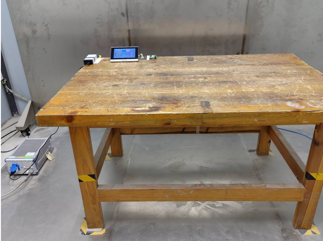
Conducted Emissions Side View- PoE power Supply mode
