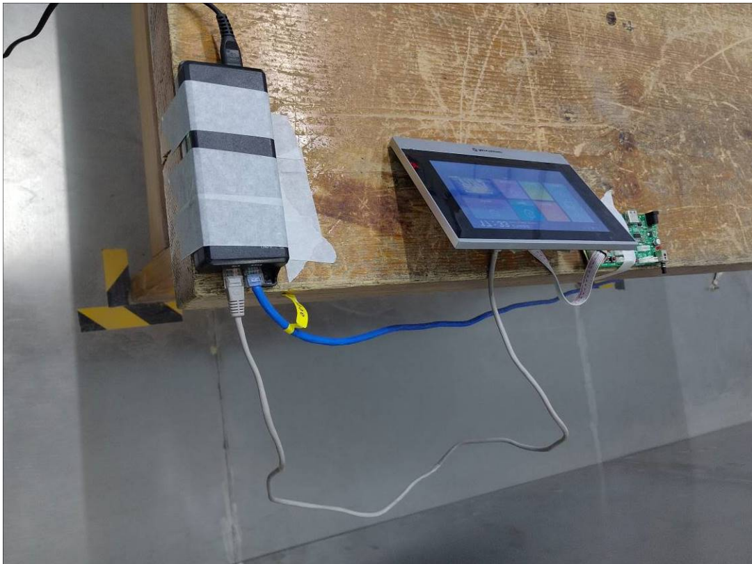
Conducted Emissions Side View- PoE power Supply mode
