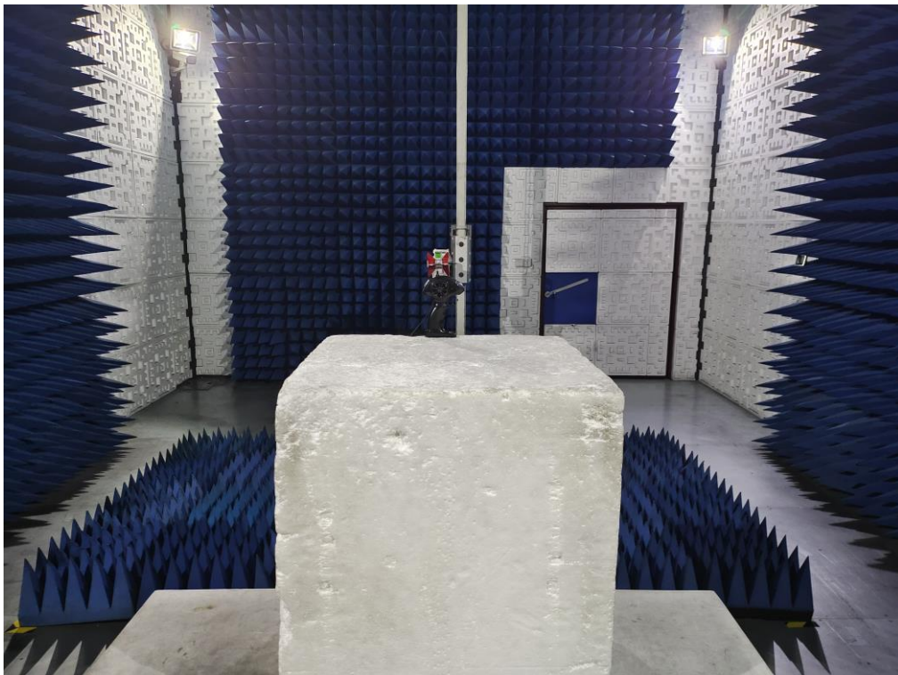
RADIATED EMISSION TEST SETUP ABOVE 1GHz
