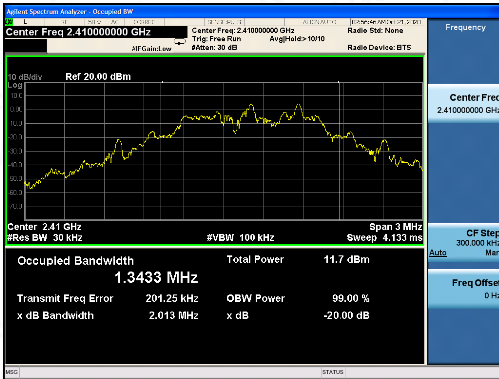
TEST PLOT OF BANDWIDTH FOR LOW CHANNEL
