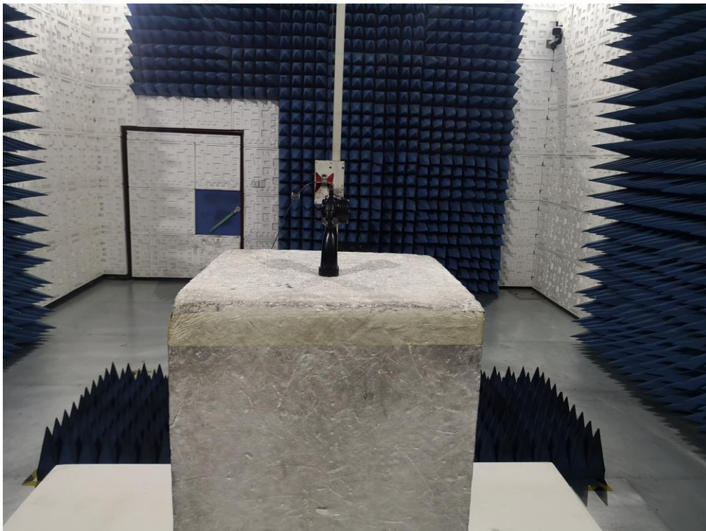
FCC RADIATED EMISSION TEST SETUP ABOVE 1
