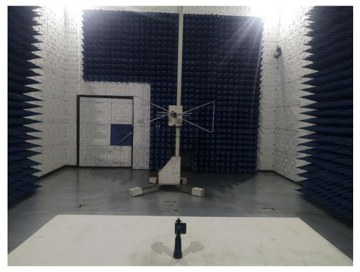
FCC RADIATED EMISSION TEST SETUP ABOVE 1
