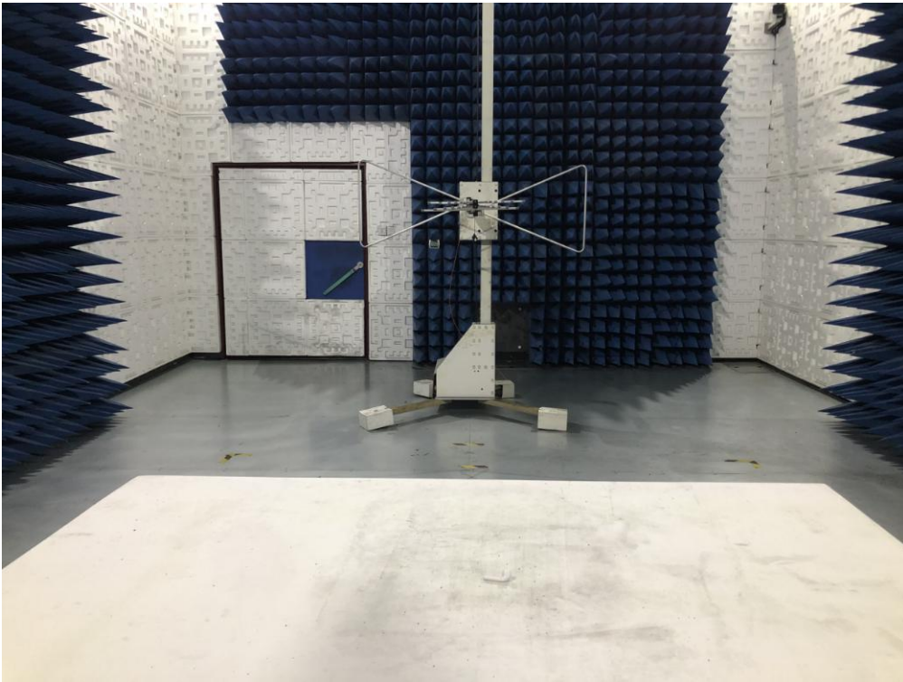
RADIATED EMISSION TEST SETUP ABOVE 1GHz
