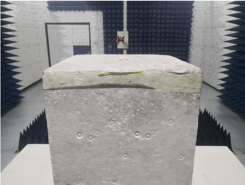
RADIATED EMISSION TEST SETUP ABOVE 1GHz
