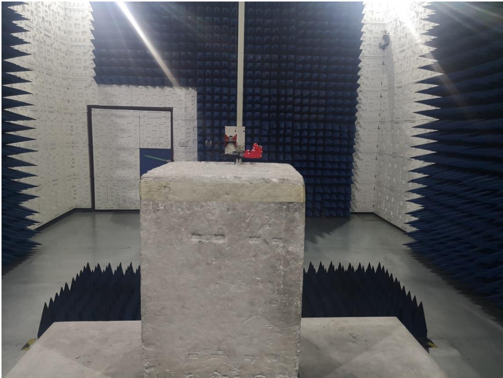
RADIATED EMISSION TEST SETUP ABOVE 1GHZ
