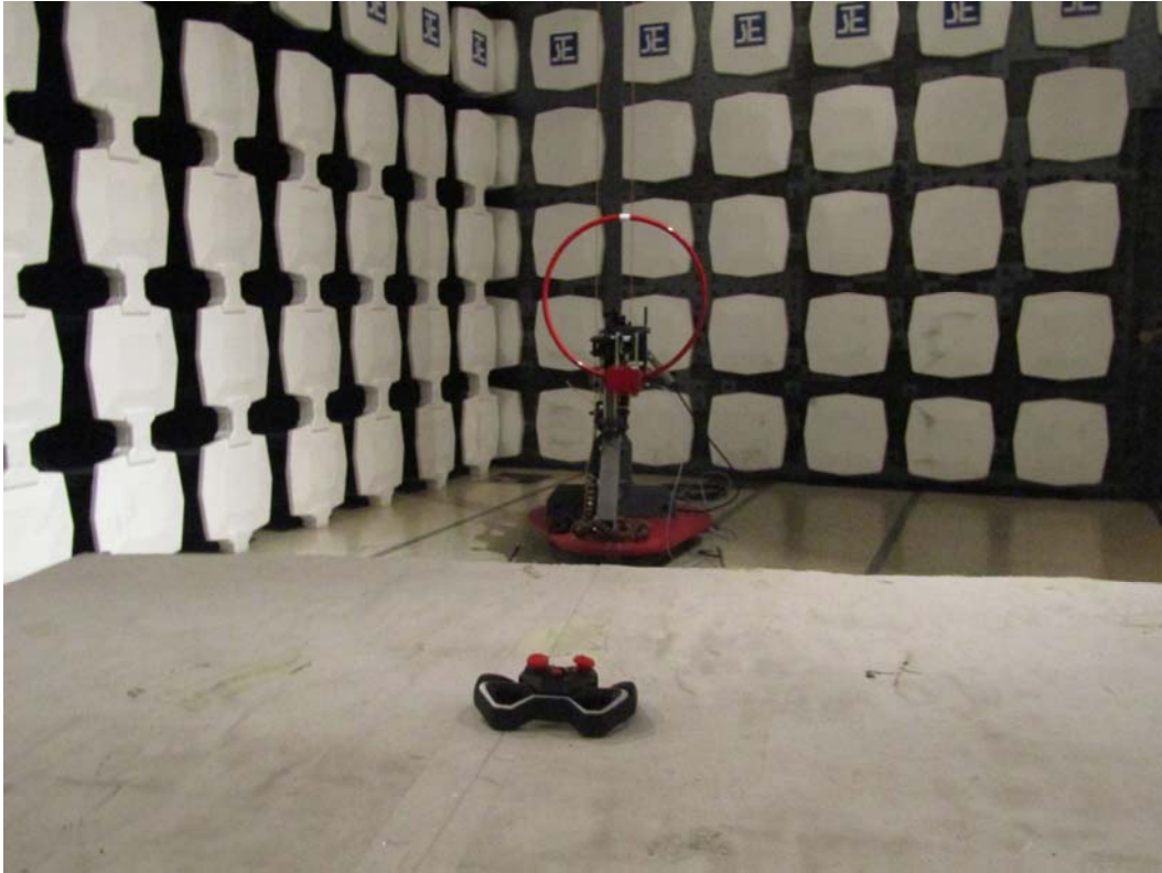
Measurement of Radiated Emission Test Set Up
