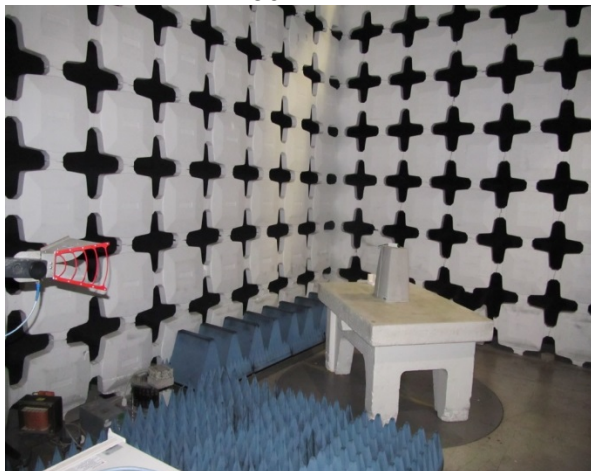
Radiated emissions test set up above 1GHz.
