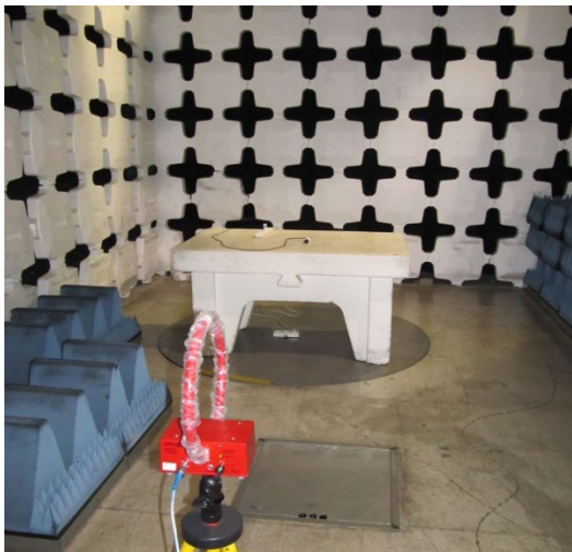
Radiated emissions test set up below 30MHz.
