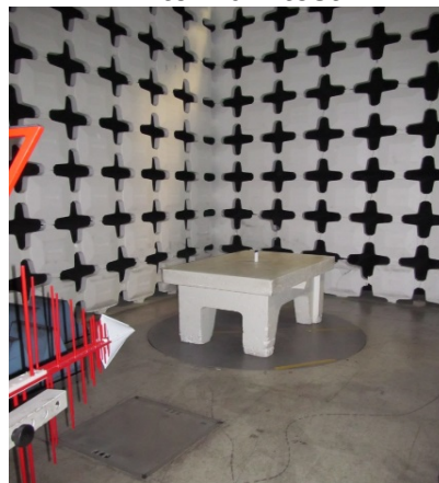
Radiated emissions test set up in 30MHz-1GHz frequency range Antenna 2 test
