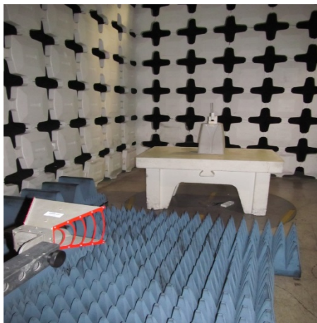
Radiated emissions test set up above 1GHz. Antenna 1 test
