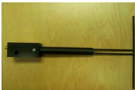
Figure 1 – MVG COMOSAR Validation Dipole
