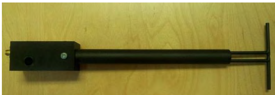
Figure 1 – MVG COMOSAR Validation Dipole
