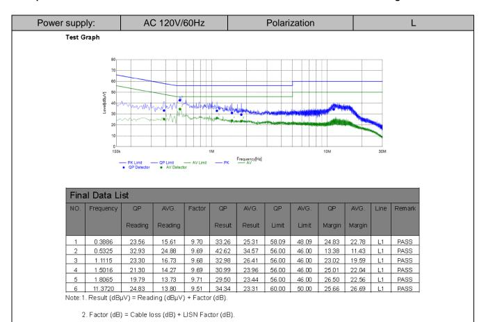
Power supply: AC 120V/60Hz Polarization N
