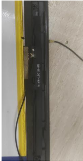
Main antenna position Conductive cloth is attached to the copper leakage area of antenna and the screen is grounded
