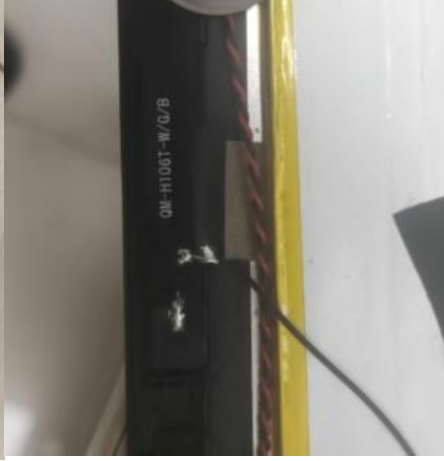
GWB Antenna Position Conductive cloth is attached to the copper leakage area of antenna and the screen is grounded
