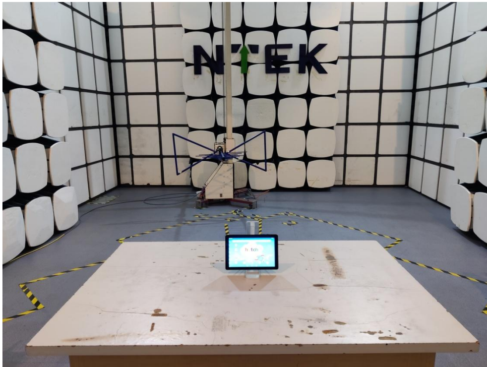
Radiated Measurement Photos(30MHz~1GHz )
