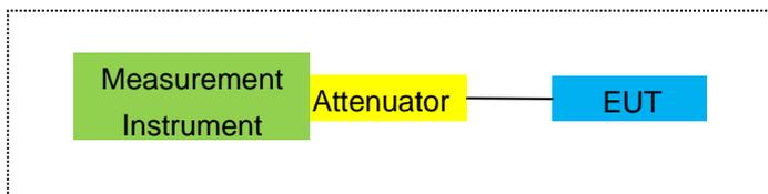
For Peak-to Average Ratio, Occupied Bandwidth, Conducted Band edge and Conducted Spurious Emission
