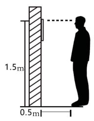
When using the device for registration and identification, the installation location of the device must remain unchanged. If you really need to move the device, you must keep the installation height consistent. If it is inconsistent, it may affect the recognition effect. It is recommended that the distance between the face and the machine at the time of registration is 0.5-0.8 meters.
