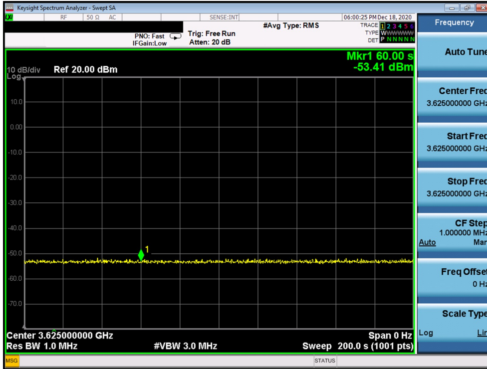
Plot 18. Conducted Measurement – No RF transmission in entire band at anytime (WINNF.FT.C.HBT.9)
