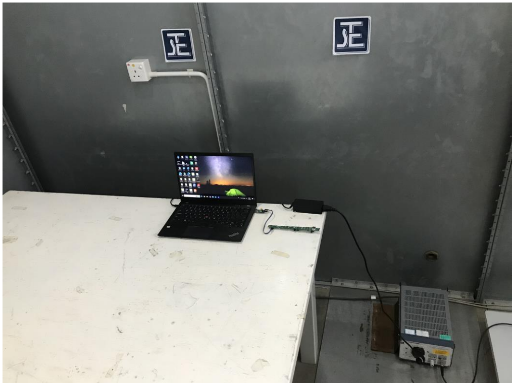
Measurement of Conducted Emission Test Set Up
