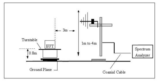
(C) Radiated Emission Test-Up Frequency Above 1GHz
