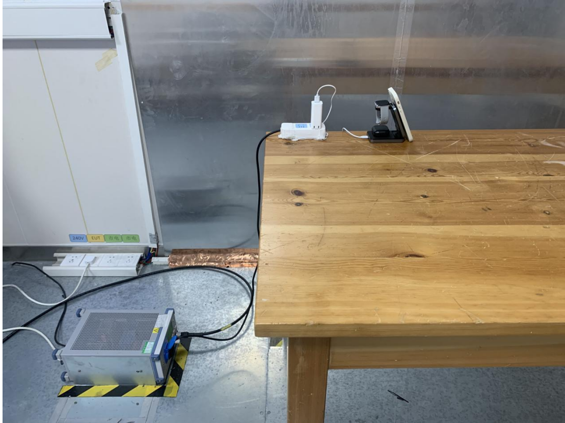
Conducted emission test setup
