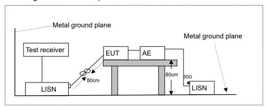
LISN: Line Impedance Stabilization Network
