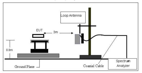
(B) Radiated Emission Test-Up Frequency 30MHz~1GHz
