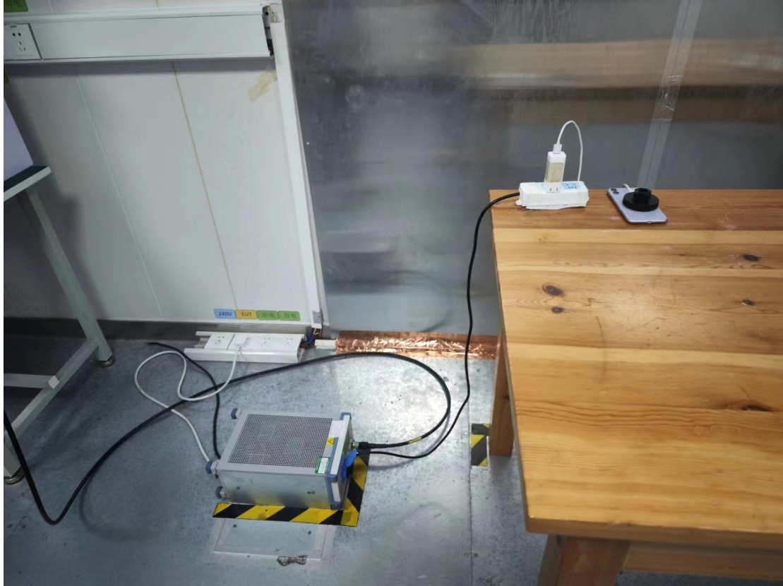
Conducted emission test setup
