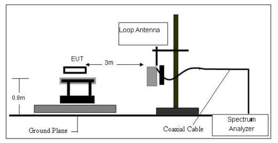
(B) Radiated Emission Test-Up Frequency 30MHz~1GHz
