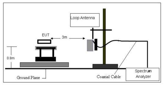
(B) Radiated Emission Test-Up Frequency 30MHz~1GHz
