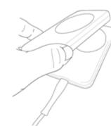
Press the power button and place it on the BeraShield Charger. It automatically sticks to the position for the best wireless charging efficiency with strong internal magnets. The red LED turns on when wireless charging is started.
