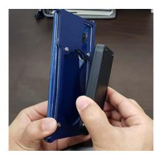
**3.** Attach the auxiliary battery to the phone case. (The phone case and battery are magnetically attached.)
