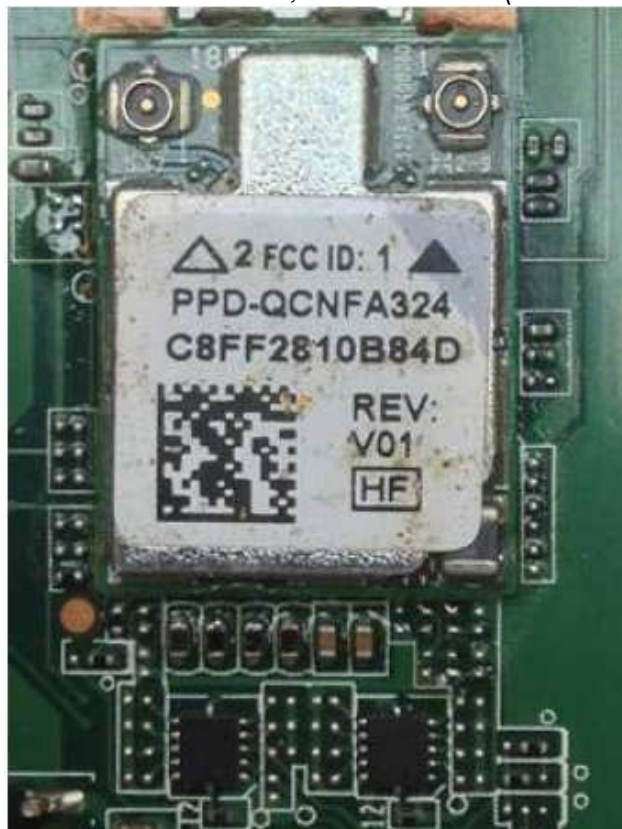
Figure 54 Medical Grade Mobile Tablet PC, Internal View (Wireless Module)
