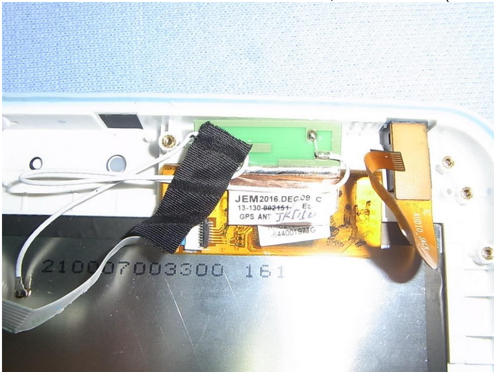
Figure 41 Medical Grade Mobile Tablet PC, Internal View (GPS Antenna)
