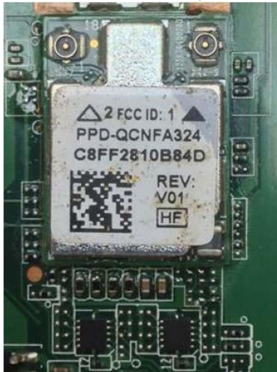
Figure 31 Medical Grade Mobile Tablet PC, Internal View (Wireless Module)
