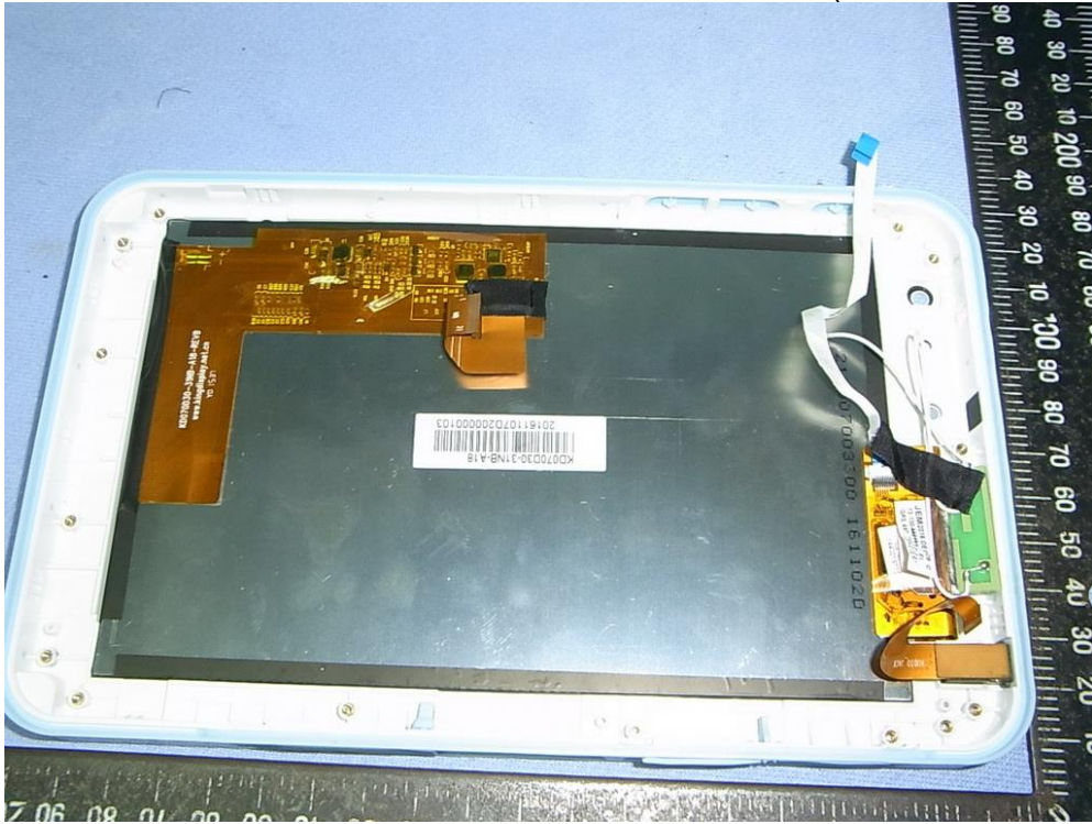
Figure 42 Medical Grade Mobile Tablet PC, Internal View (LCD Panel, Back View)
