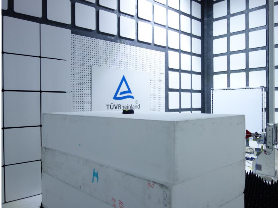
Photograph 3: Set-up for Spurious Emissions (Back View 1)
