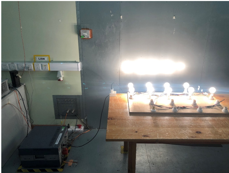
Photograph 3: Set-up for Conducted Emissions ON AC mains
