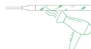
**4** Strip off the protective film; (Notice: Do not peel off the tape under the film.)
